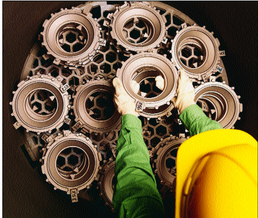
Fig. 2 — In hot isostatic pressing, or HIP, elevated temperatures and isostatic pressure are simultaneously applied to components for a precisely controlled time. The heat- and pressure-treating process can be used to reduce or eliminate voids in castings through creep and diffusion bonding. These Ti-6Al-4V seal housings are being loaded into a HIP vessel at Howmet Castings, Whitehall, Mich. HIP'ing will reduce microshrinkage in the castings. Photo courtesy of Howmet Castings.
